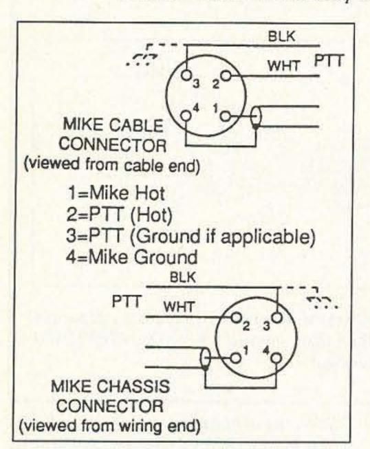
Figure 5. Microphone jack wiring to the SSTV interface.
